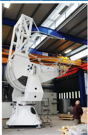
Prof. Hans Paar inspects the 3.5 m POLARBEAR telescope which will be used for the search for the existence of primordial gravitational waves in the 3 Kelvin Cosmic Microwave Background radiation.
