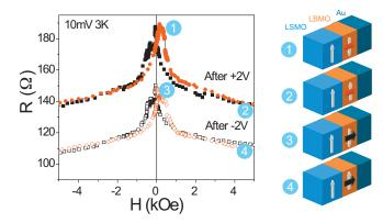
FIG. 9. (Color) Four state resistance of a tunnel junction composed of a biferroic tunnel barrier ( $La_{0.1}Bi_{0.9}MnO_3$ ) between a ferromagnetic electrode of  $La_{2/3}Sr_{1/3}MnO_3$  and a nonmagnetic electrode of gold. The states 1–4 correspond to the magnetic (white arrows) and electric (black arrows) polarizations represented on the right side of the figure. From Gajek *et al.*, 2007.
