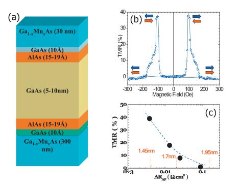
FIG. 12. (Color) Spintronics with semiconductors illustrated by experimental results (Mattana et al., 2003; Fert et al., 2007) on the structure represented on the right side and composed of a GaAs layer separated from the GaMnAs source and drain by tunnel barriers of AlAs. (a) MR curve at 4.2 K showing a resistance difference of 40% between the parallel and antiparallel magnetic configurations of the source and the drain. (b) MR ratio as a function of the resistance of the tunnel barriers.
