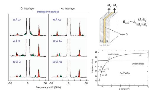
FIG. 5. (Color) Left-hand side: Representative BLS spectra from spin waves in Fe/X/Fe, where X=Cr and Au (Grünberg *et al.*, 1986). The plot on the right-hand side displays the mode frequencies as a function of the interlayer exchange parameter  $J_1$  (Barnas and Grünberg, 1989), where the theory is represented by the solid lines.
