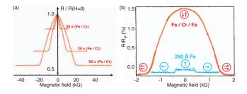
FIG. 9. (Color) GMR effect in (a) a multilayer and (b) a double layer of Fe interspaced by Cr. In (b) the AMR of a 250-Å-thick film of Fe is also shown for comparison.
