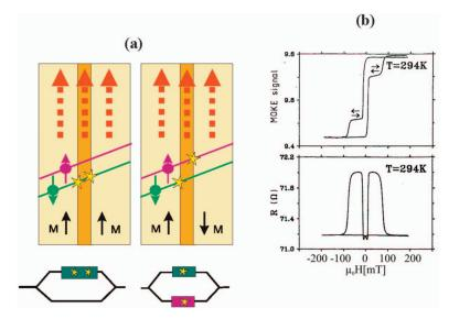
FIG. 10. (Color) (a) Explanation of the GMR effect: spin-dependent electron scattering and redistribution of scattering events upon antialignment of magnetizations. The antiparallel alignment can be obtained by antiferromagnetic coupling, like in Fig. 9, or due to hysteresis effects, like in (b).
