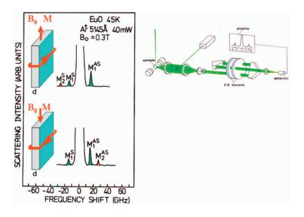
FIG. 1. (Color) Right: Schematic of a Brillouin light scattering (BLS) spectrometer used for the detection of spin waves. Spectra of scattering from bulk spin waves (marked with green) and DE surface spin waves (red) are seen on the left. For the upper and lower parts on the left, the field  $B_0$  and magnetization *M* have been reversed. From Grünberg and Metawe, 1977.
