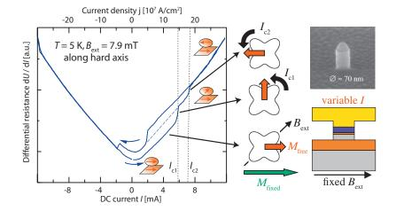
FIG. 12. (Color) Two-step CIMS in Fe/Ag/Fe. Four energetically nearly identical states give rise to two-step switching (Lehndorff *et al.*, 2007).
