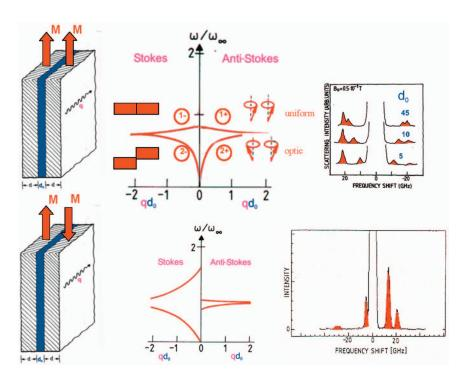
FIG. 3. (Color) Coupled DE modes in magnetic double layers for parallel (upper part) and antiparallel (lower part) alignment of the magnetization M (Grünberg, 1989). Calculation in the dipolar limit. For the spectrum in antiparallel alignment, a sample showing AF coupling (to be discussed later) was used. Peak positions are mainly due to the dipolar interaction with small corrections due to exchange coupling.
