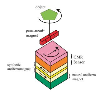
FIG. 14. (Color) Working principle of a GMR spin-valve-type sensor, used here for measurement of rotational angles.
