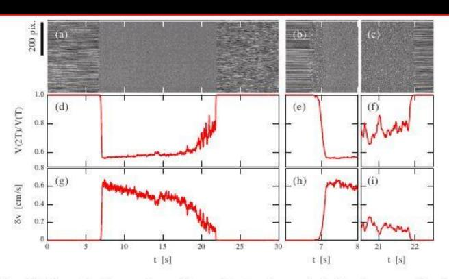
FIG. 2. (Color online) Time-stacked line-scan images of the speckle pattern for an avalanche (a) and zoom-ups of it turning on (b) and turning off (c). The middle row shows the corresponding variance ratios, which are transformed into the fluctuation speeds in the bottom row.
