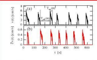
FIG. 3. (Color online) (a) Average and (b) fluctuation speed time traces for independent observations with the same sand flux  $Q = 0.07 \, \text{g/s}$ . The on and off times,  $T_{\text{on}}$  and  $T_{\text{off}}$ , for the nth avalanche event are defined as shown.
