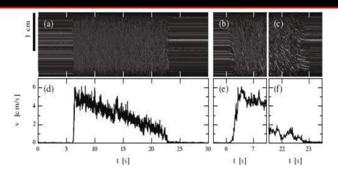
FIG. 1. Time-stacked line-scan images of the surface of the heap for an avalanche (a) and for zoom-ups of it turning on (b) and turning off (c). Sand grains appear as bright lines with slope proportional to their speed down the channel. The slope is measured by locating the maximum of the cross-correlation function for consecutive time snapshots. The bottom row shows the flow speeds extracted from the corresponding images above.
