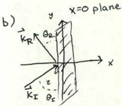
perfectly conducting surface, 100% reflecting
