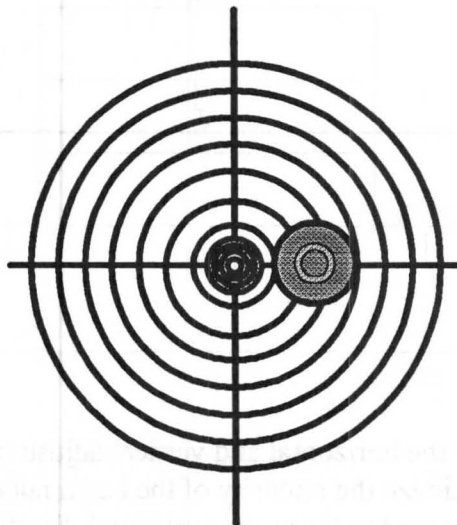
Figure IV-15: Target Image of Laser Through Misaligned Detector
