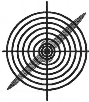
Figure IV-11: Image of Target for Lens Adjustments
